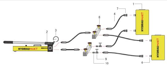
**Set-up two:** Two-way hand pump + Two manifolds + Six hoses + Two double acting hydraulic cylinders With 2- or more-port manifold, the system allows simultaneous lift and descent of several double acting cylinders. Throttle valve installed on the outlet port of manifold regulates the flow of hydraulic fluid to or from the cylinders, so as to control the lift and descent of each cylinder and maintain horizontal movement of load.
