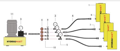
**Set-up Three: One-way electric pump + Manifold + Five hoses + Four single acting cylinder** With 4- or more- port manifold, the system allow simultaneous lift of several single acting cylinders. Throttle valve regulates the flow of hydraulic fluid to or from the cylinders. One- way valve allows safety holding of load in lifting applications.
